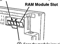
Snap the module into place by pushing it down.
